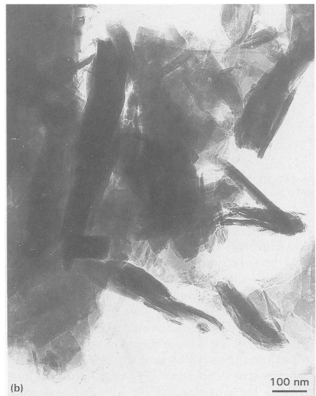
Figure 9 TEM photographs of (a) bent and broken crystals in the Caobar kaolinite sample pressed at 0.85 GPa; (b) kaolinite sample pressed at 2.0 GPa.
